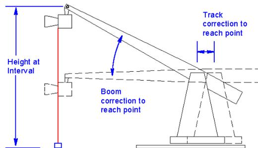
In our case, for the first point, 30cm, we had to boom up to 176cm above the ground. Once we did this, and corrected the track forward to return to the laser dot, we found we had a boom angle of +6.840 degrees and a truck forward of -1.961cm. These are the correction coefficients the Kuper would have to use if you told it to raise 30cm straight up.
