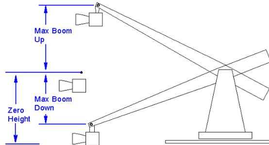
Calculate the range above and below zero and break it into 3 or 4 intervals each side of zero. On the rig used in this example, the upper excursion was 133cm, and the lower excursion was 138cm.
