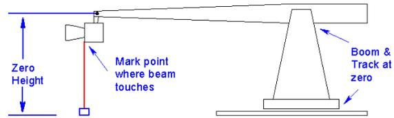
**Carefully zero your track and boom and take one last measurement of the height of your reference point.** For our CNC rig example, the zero height was an even 146cm. Add this zero height to each interval to calculate the how high your reference point would be above the floor at each of those intervals.
