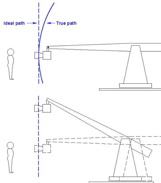
That's the basis of the Kuper "virtual axis" strategy. You describe the machine mathematically to the Kuper software, and the software then continuously calculates the "tweaks" necessary to keep the camera moving in an idealized line.
