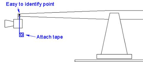
Measure the boom height at zero. Then exercise the boom to find its upper and lower range limits. On some machines, you may have to move down the track and work past the track end or even remove the camera head to find the practical lower limit. You're going to want to include any boom excursion that you're likely to use in real-life in the table.
