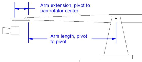
For our example rig, the working length of the arm is 243.8cm, and the extension is 30.5cm.
